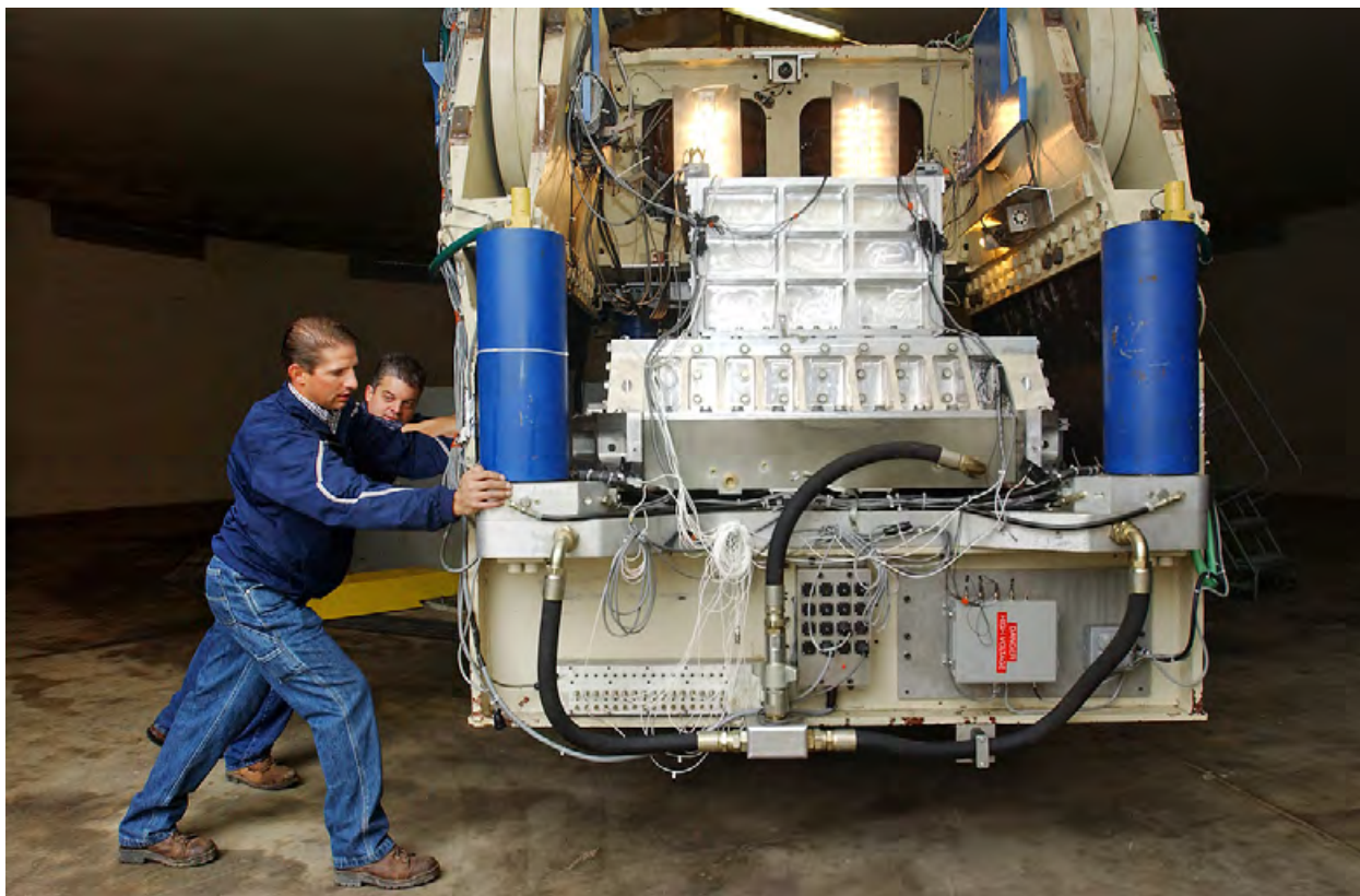
Chad Justice, left, and Tom Kohnke ready a geotechnical centrifuge at the UC Davis Network for Earthquake Engineering Simulation site. The centrifuge is the largest in the U.S. and among the largest in the world.
